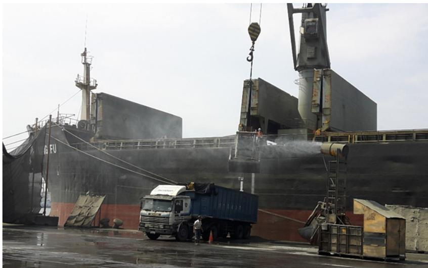
▲ Fugitive particulate matter is released while unloading cement clinker in port zones
