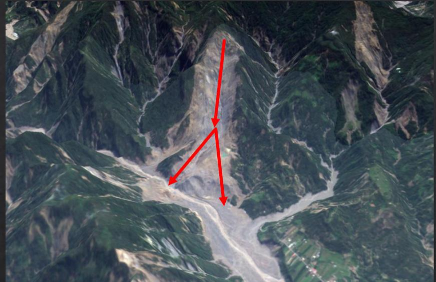
◇ The material runs into the main channel, but could not form the landslide dam
